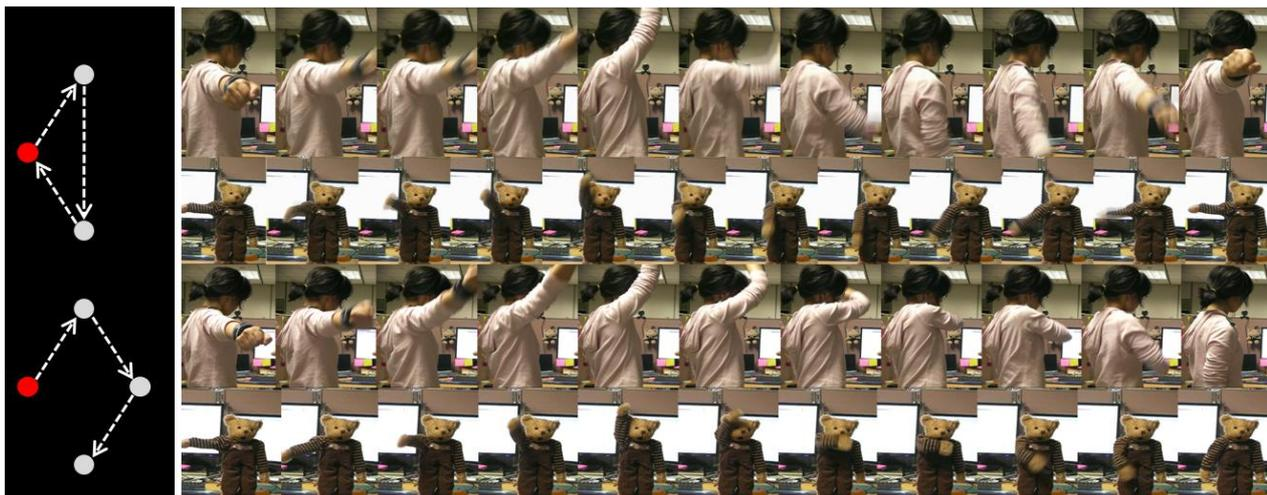
Fig. 7. Human demonstration with accelerometers for robot imitative learning. The red circle means the starting position of a continuous gesture.
