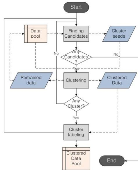
Figure 2. Flow chart for incremental QT clustering. Dotted lines represent the flow of primitive instances, and solid lines represent the process flow.
