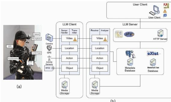
Figure 3. The Life-log system. (a) A user wears a sensor network that includes a camera, microphone, GPS device, RFID glove and accelerometers. (b) Process flow of the LLM system.
